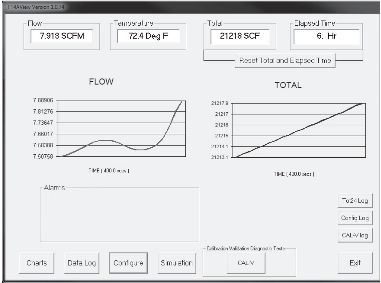
Fig. 3.1: FT4A View™ Main Screen
